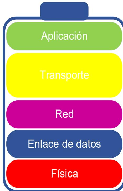
FIGURA 2(CAPAS DEL MODELO TCP/IP)
